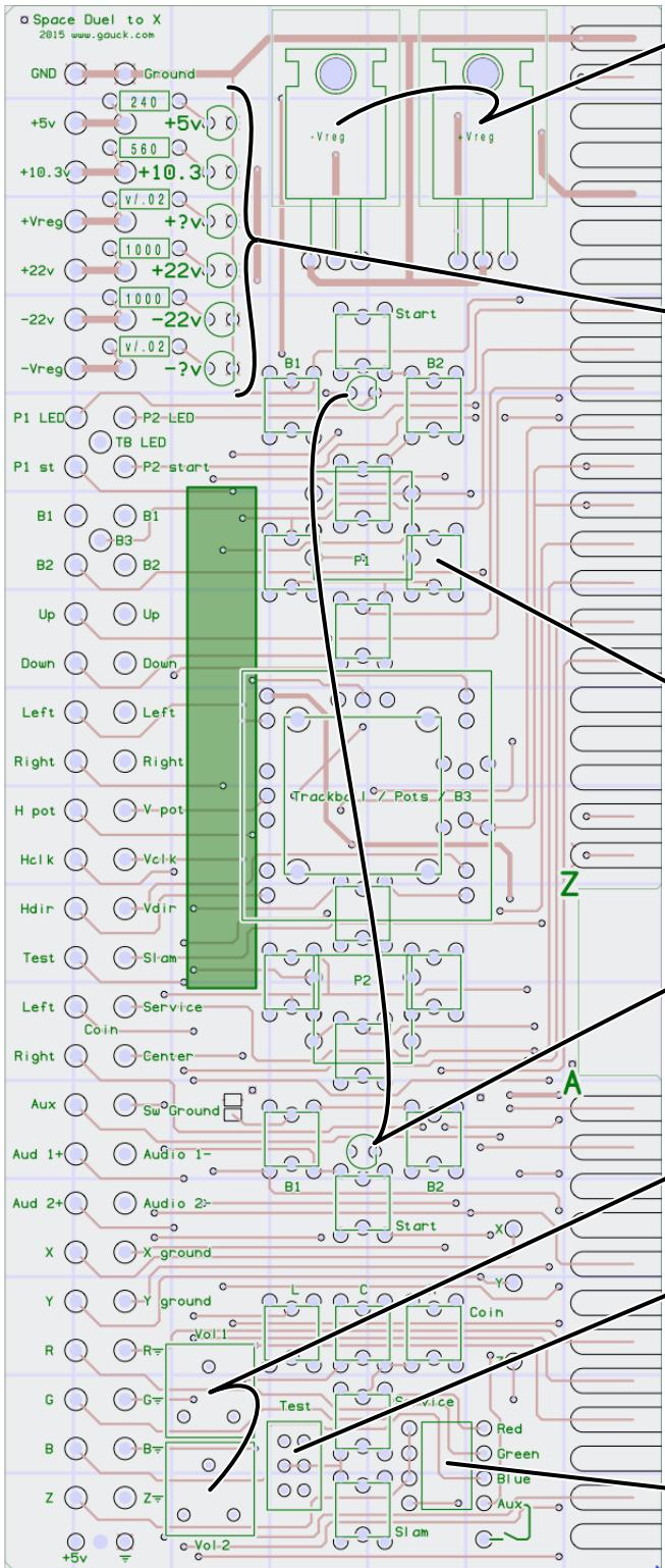
Voltage regulators (optional): supply user-selectable voltages at the holes on the left edge of the VTBA. The -Vreg is connected to -22v and GND, and will accept a 79xx series TO-220 package. Fitting a 7905, for example, will supply -5v to the -Vreg holes. The +Vreg supplies positive voltages to the +Vreg holes by fitting a 78xx series part.
