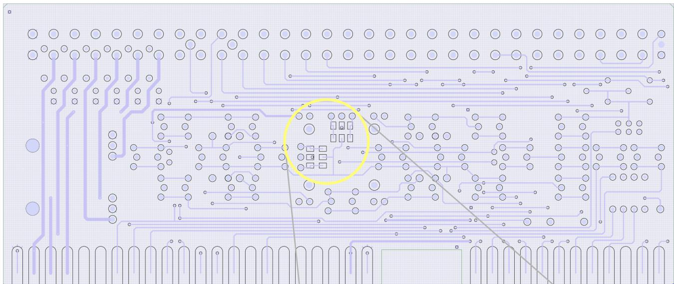
These six pads are arranged to allow one end of the joystick's potentiometer to be connected to ground, and then other end connected to +5v.
