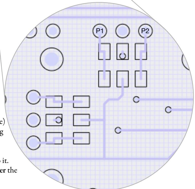
Test the first axis. If your player moves opposite from the desired direction then redo both solder blobs to change from one configuration to the other. If your player moves along the wrong axis (up/down instead of left/right) then swap the wires between 'V pot' and 'H pot.' Once it's sorted, rotate the board 90° clockwise and repeat for the other pot.
